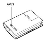
Set AVLS to LIMIT. The volume is kept at a moderate level, even if you try to turn the volume above the
